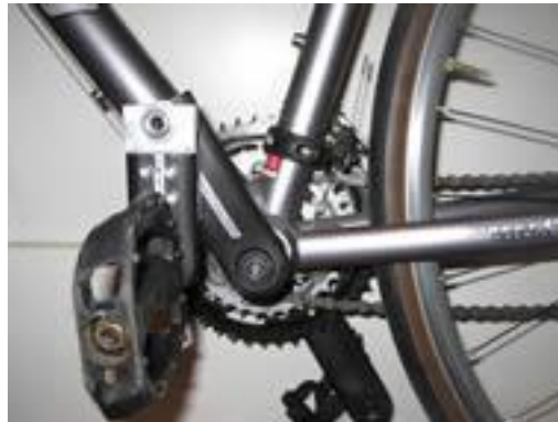
Figure 7: Pivoting Crank Arm
